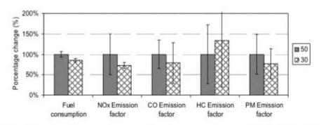
Figure 7. Modification of emissions and fuel consumption in the studied urban route when the speed limit is reduced to 30 km h<sup>-1</sup>
